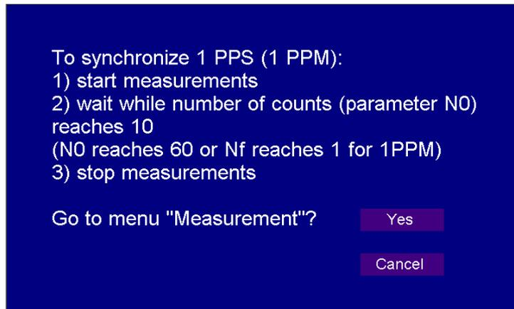
Figure 29. Screen with information about time scale adjustment procedure
