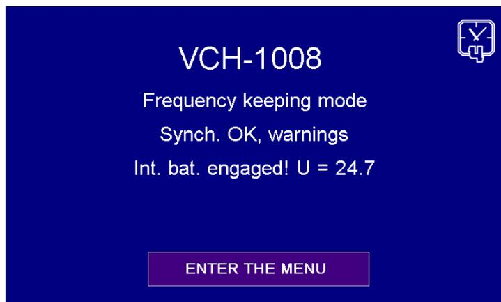
Figure 35. Status screen with information about accumulator’s discharging
