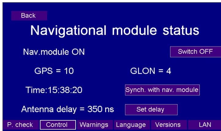
Figure 30. Submenu “Navigational module status”, normal operation
