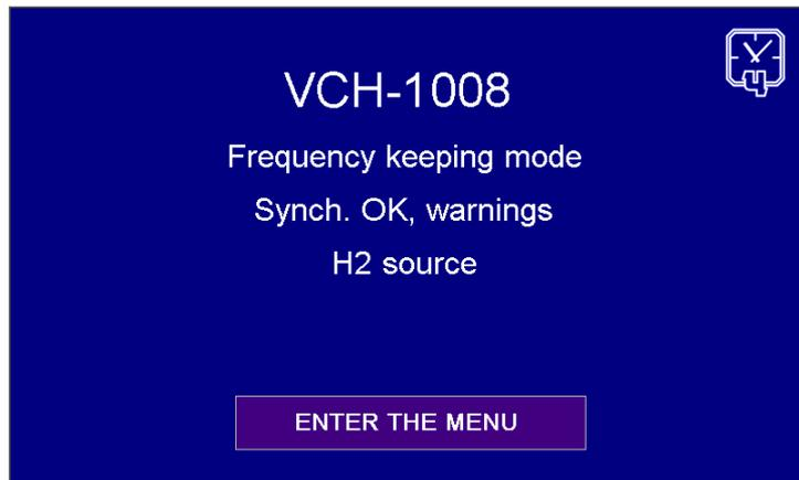
Figure 4. Status screen informing about normal operation with warning
