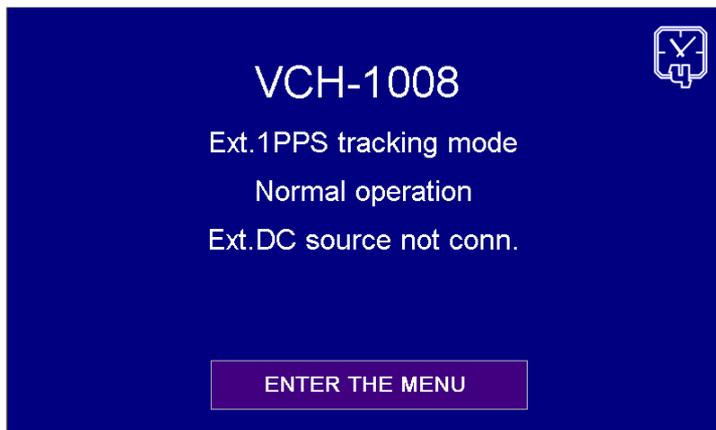
Figure 25. Example of status screen in case of measurement process is in progress and synchronization source is external 1 PPS
