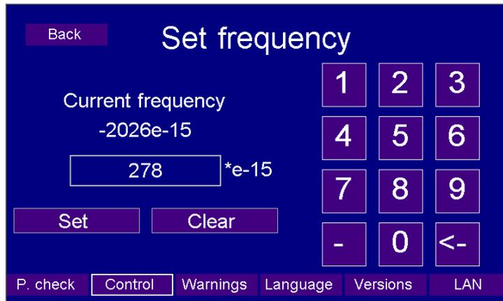
Figure 15. User interface for output signal frequency setting
