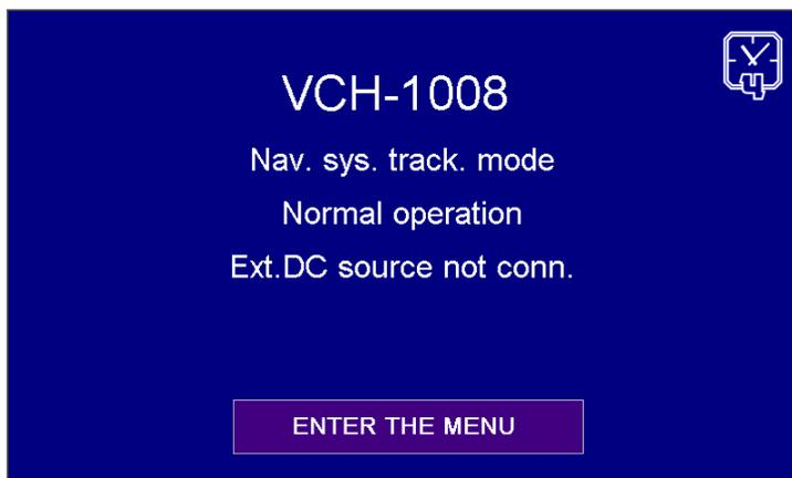
Figure 26. Example of status screen in case of measurement process is in progress and synchronization source is navigational module
